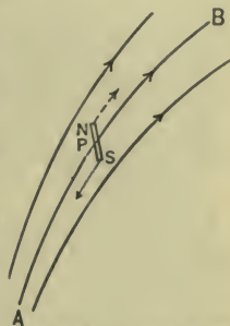
FIG. 815.—Lines of magnetic force, and the forces acting on a small magnet.
