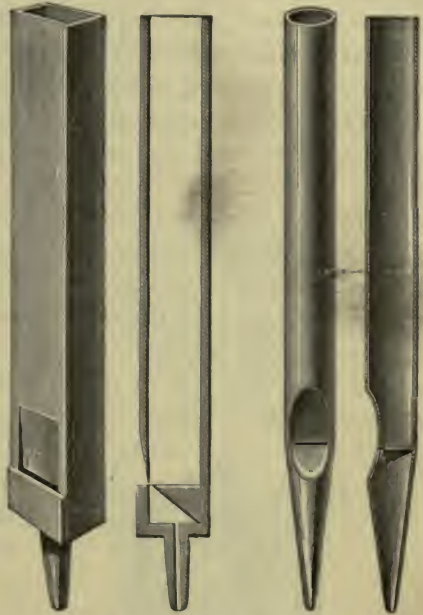
FIG. 161. — Section of an ordinary organ pipe.
