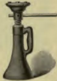
FIG. 68. — Screw and nut lifting Jack.
