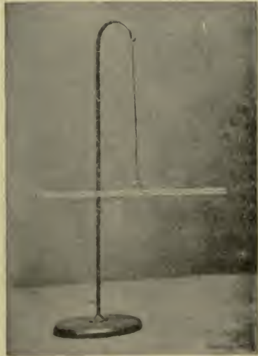
FIG. 330. — A glass rod suspended in a stirrup so as to be free to turn.
