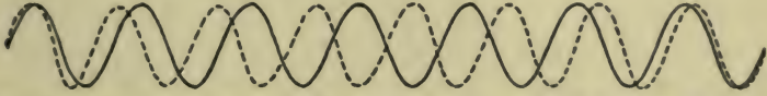
FIG. 154. — Diagram showing origin of beats. The two vibrations have frequencies whose ratio is 7 : 8.
