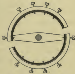
FIG. 114.—Balance wheel of a watch; the inner portion of the rim is iron; the outer is brass.
