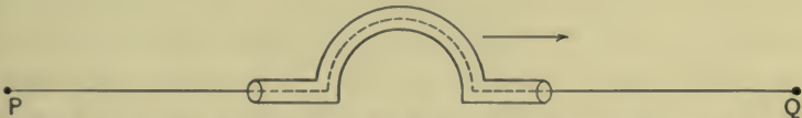
FIG. 149. — A cord, over which has been slipped a bent tube, is stretched between P and Q .
