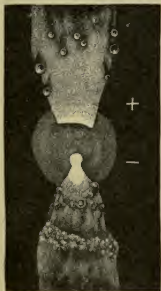
FIG. 853. — The electric arc between two carbon poles.
