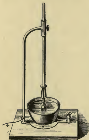
FIG. 379. — A simple form of silver voltameter.
