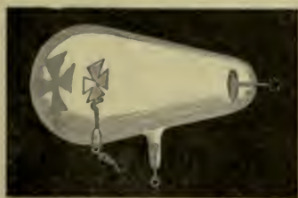
FIG. 383.—Shadow of maltese cross produced by cathode rays.
