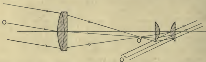
FIG. 251.—Astronomical telescope: O is source at an infinite distance; O' is image formed by object glass; O'' is virtual image formed at an infinite distance by the eyepiece.
