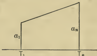
FIG. 11. — Special case, when the quantity whose mean is desired is varying at a uniform rate.
