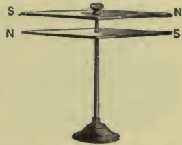
FIG. 863. — An astatic combination of magnets.
