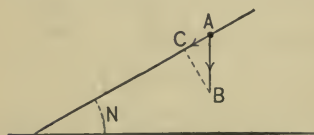
FIG. 18.—The component along an inclined plane of a vertical vector \overline{AB} is \overline{AC} \sin N .
