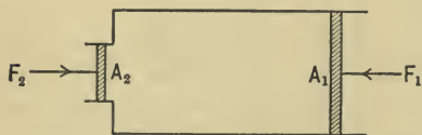
FIG. 78. — A fluid is inclosed in a vessel closed by two pistons of different areas. Neglecting gravity, \frac{F_1}{A_1} = \frac{F_2}{A_2} , Pascal's Law.
