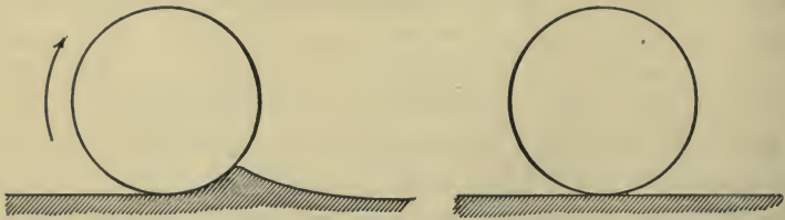
FIG. 59. — As a body rolls on a plane surface, both are deformed slightly.
