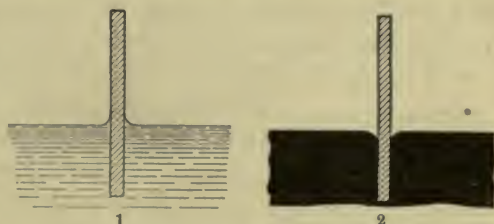
FIG. 91. — Capillary action when a solid plate is dipped in a liquid: (1) when the liquid wets the solid; (2) when the liquid does not.
