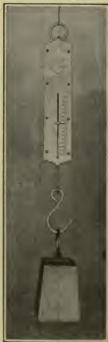
FIG. 29. — Spring Balance used for measuring weights.
