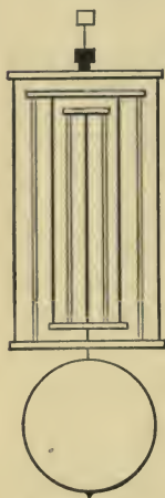
FIG. 113. — Compensation "grid-iron" pendulum. The single black lines represent iron rods; the double lines brass ones.
