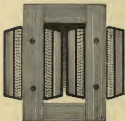
FIG. 419 a.—Section of a commercial transformer.
