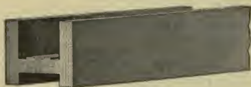
FIG. 73. — Standard form of metre bar, with the divided scale along its neutral section.
