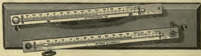
FIG. 110. — Rutherford's maximum and minimum thermometers. The former contains mercury, the latter alcohol.
